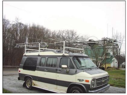
putting the 6M antenna at a few inches less than 30' above ground when in the up position. It is removed for travel.
